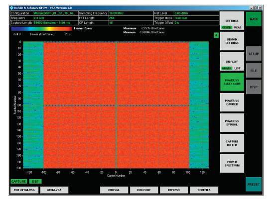
The diagram shows the power of each carrier and symbol of the received frames in dBm for each carrier. The values are colorcoded in accordance with a table of colors that is displayed in the upper area of the measurement window.
