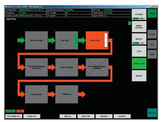
The signal flow diagram describes the current measurement status in detail. It also offers information about the area in which the signal to be analyzed is faulty or deviates from the settings. The signal flow diagram is thus a powerful tool for troubleshooting problems in the modulation of the signal. In this example, the pilot cells of the signal do not match the configurations. Unused blocks are crossed out.
