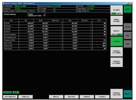
The summary of results offers a quick overview of the most important numeric measurement results. The calculation includes all analyzed frames in the capture buffer.
