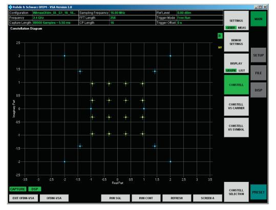
The constellation diagram shows the in-phase and quadrature components over the entire area of the measured input data. It can be displayed either for all carriers or for selected carriers. Color coding makes identification of the different modulation formats easy.
